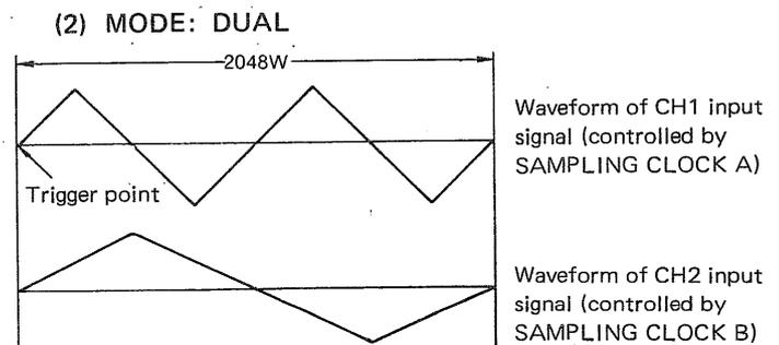
CH1 and CH2 input signals are same, but SAMPLING CLOCK A is set to twice the SAMPLING CLOCK B setting.
