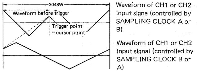
SAMPLING CLOCK A (or B) is set to twice the SAMPLING CLOCK B (or A) setting.
