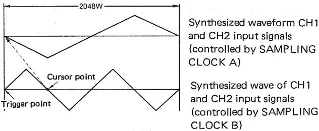
SAMPLING CLOCK B is set twice the SAMPLING CLOCK A setting.
