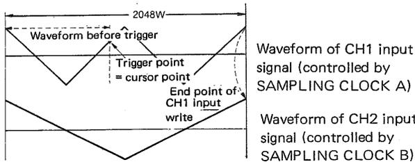
CH1 and CH2 input signals are same, but SAMPLING CLOCK A is set to twice the SAMPLING CLOCK B setting.
