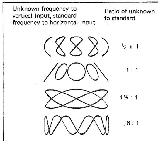
Fig. 30 Lissajous' patterns used for frequency measurement
