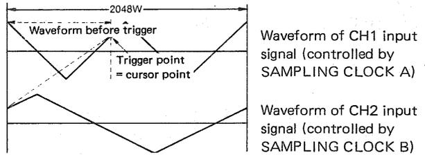
CH1 and CH2 input signals are same, but SAMPLING CLOCK A is set to twice the SAMPLING CLOCK B setting.
