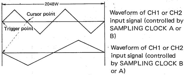
SAMPLING CLOCK A (or B) is set to twice the SAMPLING CLOCK B (or A) setting.
