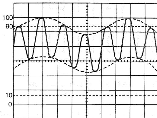
Signal containing undesired component
